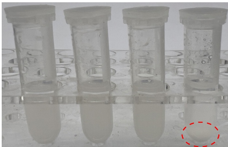
Figure S6. Photographs of BQRGP1-4 dispersed in ultrapure water for 24 h. It can be observed that there was no precipitation for BQRGP1-3, whereas BQRGP4 precipitated slightly.
