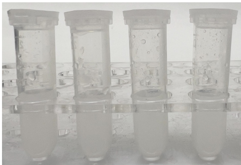
Figure S10. Photographs of BQRGP1-4@HMON-SNO dispersed in ultrapure water for 24 h. BQRGP1-4@HMON-SNO were all dispersed well without any precipitation.
