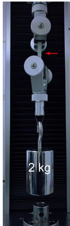
Figure S14. A rectangular sample of B 80 A 20 -M 6 hydrogel (0.2 x 8 x 60 mm) lifted 2 kg weights.
