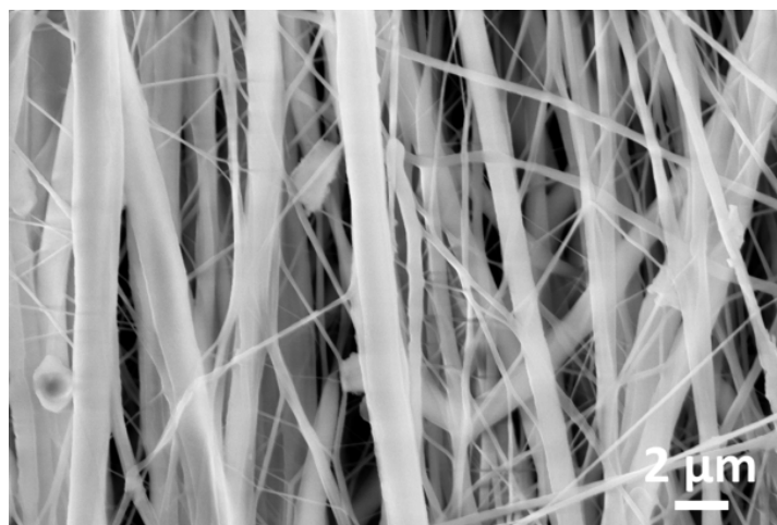
Figure S28. SEM image of PVA fibers.
