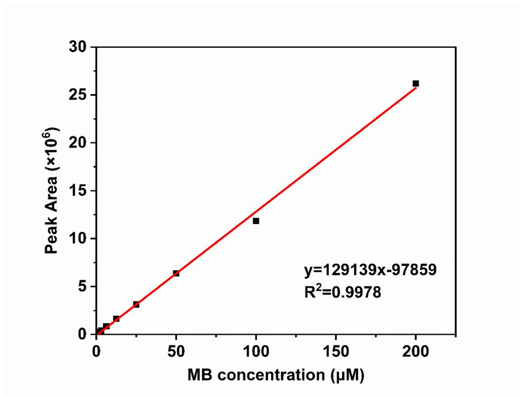
**Figure S1.** Linear relationship between various concentrations of MB (1.5–200 μM) and peak area at 665 nm *via* HPLC.
