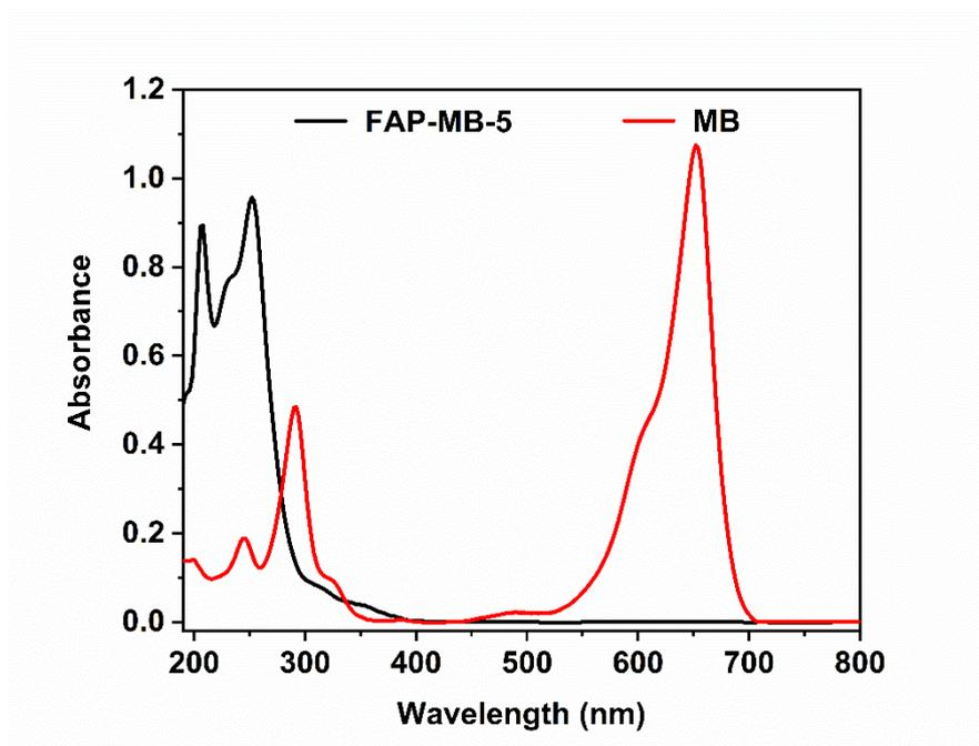
**Figure S4.** UV-vis absorption spectra of FAP-MB-5 and MB in MeOH.
