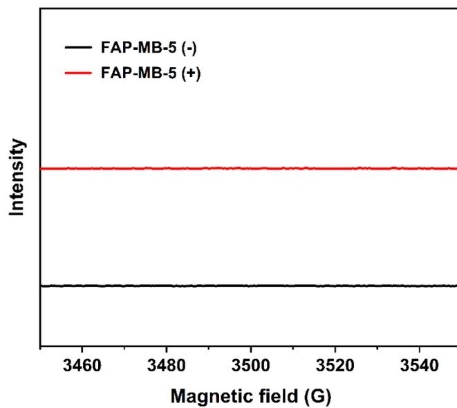
**Figure S9.** ESR spectra of FAP-MB-5 with or without irradiation. (+) and (-) refer to the treatment with or without irradiation, respectively.
