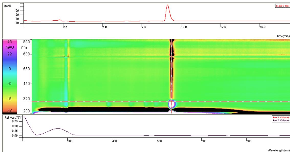
**Supplemental Figure 1.** Analytical HPLC chromatogram of cFLFLF using PDA detector.
