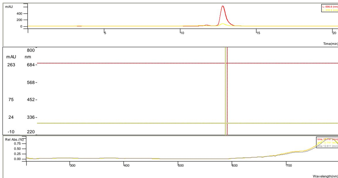
**Supplemental Figure 2.** Analytical HPLC chromatogram of cFLFLF-PEG-Cy7 using PDA detector
