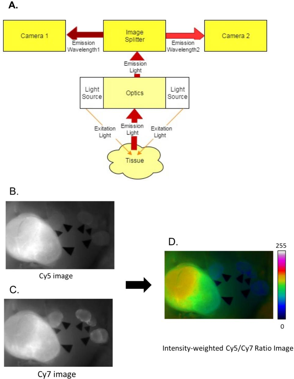
**Figure S2. Generation of Cy5/Cy7 fluorescence ratio (FR) images example in 4T1 model. (A) Optical diagram of camera instrumentation used to capture FR images. (B) Cy5 fluorescence image (C) Cy7 fluorescence image and (D) Cy5/Cy7 FR image of cervical lymph nodes shown in Fig. 4C.**
