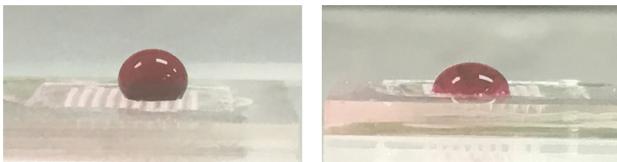
Figure S1. Images of the contact angle for the microneedle polydimethylsiloxane mold before ( left ) and after ( right ) treatment with oxygen plasma.
